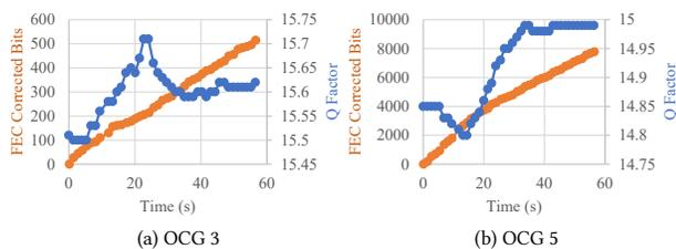
**Figure 6: QoT measurements for witness waves while adding/dropping OCG1. During the add/drop, Q factor for the witness waves is relatively constant—varying by  $\pm 0.1$ . Errors accumulate at a linear rate as expected in a live transport network; 100% are corrected with FEC while running traffic over OCGs 3 and 5.**
