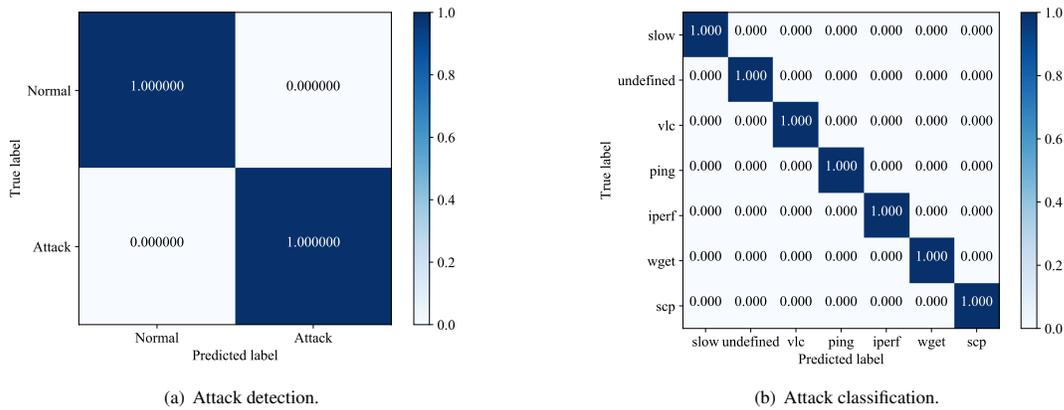
Figure 8: Confusion matrices for outlier detection and classification for multiple traffic flows comprising of familiar attack flows.
