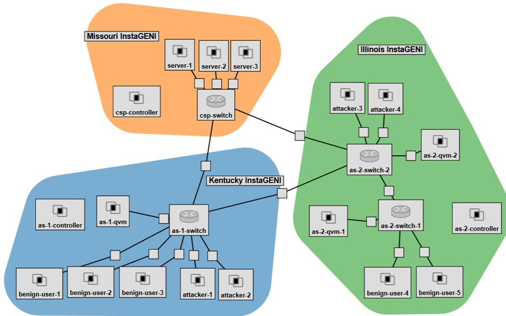
Figure 9: GENI Cloud testbed setup used to evaluate the Dolus system performance.
