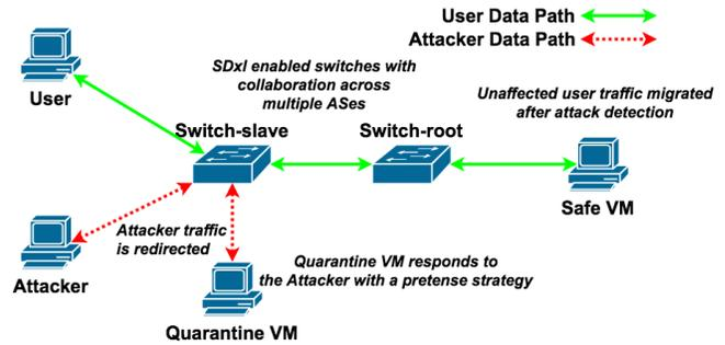
**Figure 1: Illustration of the proposed Dolus system scheme wherein the attacker is *tricked* by redirection of the attack traffic to a quarantine VM for pretense initiation, while the providers work collaboratively to block the attack traffic closer to the source side.**
