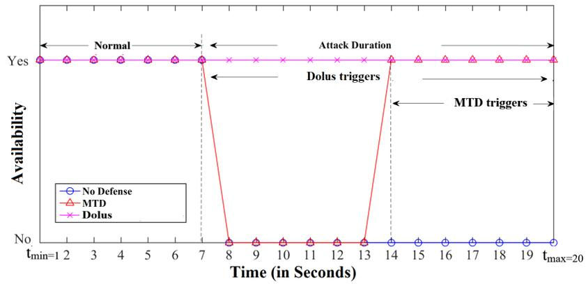
Figure 10: Comparison of the cloud service restoration time metric with cases of: no Defense, with MTD and with Dolus.
