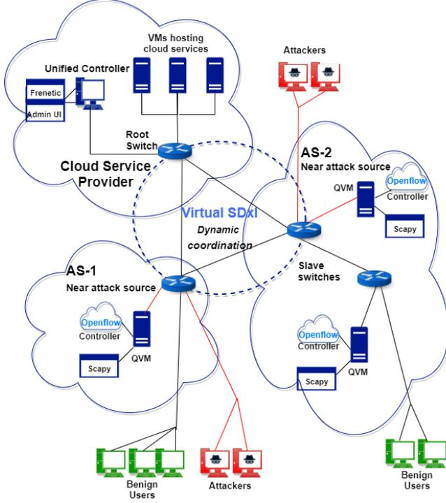
**Figure 2: Cross-domain physical setup in a Dolus system deployment to share threat intelligence for a unified controller to coordinate policy management with a federation of ASes to block attack traffic closer to the source side.**
