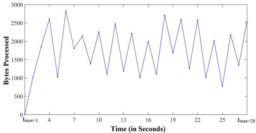
Figure 12: Traffic Processed at the root switch only shows user traffic proving that the attack traffic is redirected to quarantine VM.
