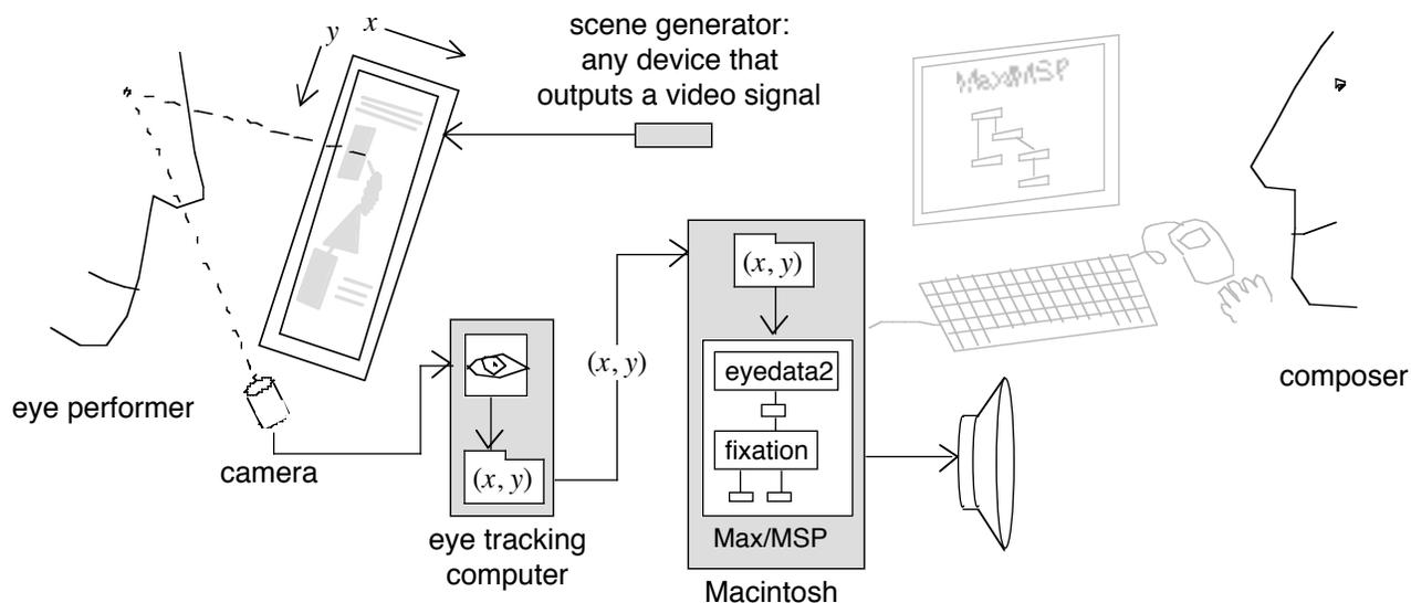
**Figure 1.** The EyeMusic system architecture is designed to get the human eye movement data to the musician in a context and format that are most useful for composing and performing. Arrows indicate the flow of data.
