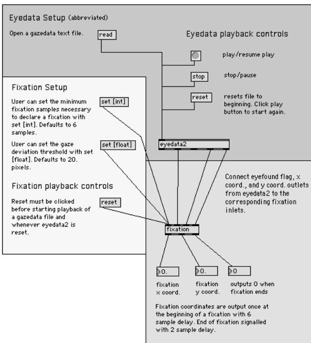
**Figure 3. To encourage the musicians to compose to the physiological phenomenon of gaze fixations, the computer scientists created a second *fixation* object that parses the eye movement data using established algorithms.**
