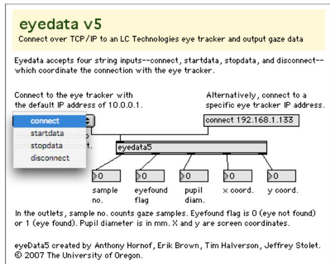
**Figure 4. The most recent version of the *eyedata* object (v5) connects directly to an eye tracker for real-time performance.**
