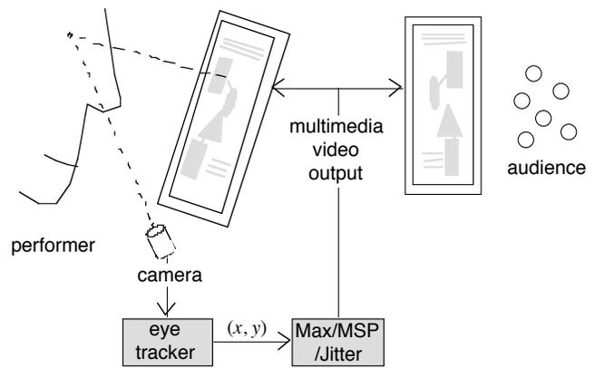
**Figure 6. The EyeMusic system configured for live performance, with the performer directly interacting with visual objects to trigger visual and musical responses.**
