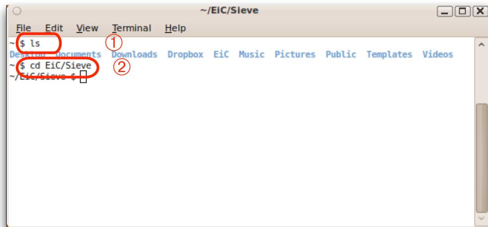
Figure 6.3: A screen shot from a session with the terminal emulator, showing how to navigate to the directory set up for the “sieve” project.
