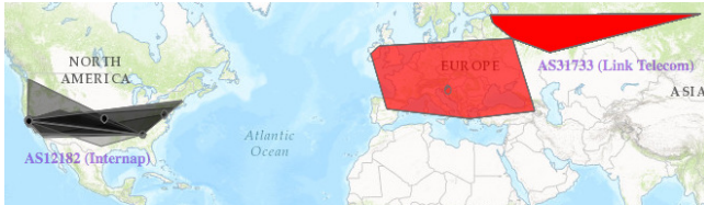
Figure 9: Footprint of BGP update events produced during (bot-tom) Link Telecom hijack scenario described in [30].
