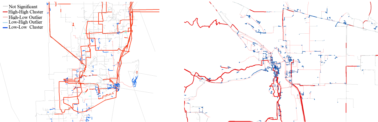
Fig. 10: A map of the downtown region for Miami (left) and Portland (right) MSAs showing fiber infrastructure labeled into various clustering regions by Moran’s I analysis.
