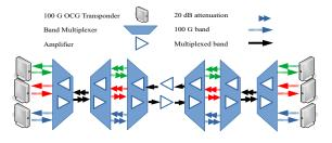
Figure 4: Configuration used in our lab-based experiments: six optical transponders, each of which generate 100 Gbps of Optical Data Unit (ODU) traffic over seven amplifiers. OptSys'21, August 23, 2021, Virtual Event, USA
