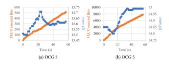
Figure 6: QoT measurements for witness waves while adding/dropping OCG1. During the add/drop, Q factor for the witness waves is relatively constant—varying by +/- 0.1. Errors accumulate at a linear rate as expected in a live transport network; 100% are corrected with FEC while running traffic over OCGs 3 and 5.
